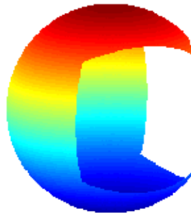
Figure 7-2: Part of a Sphere Formed by Four Rotates of a Quartic Rational
